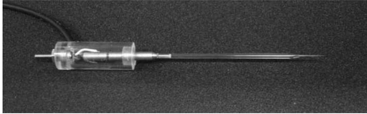
**Fig. 1.** Micro tactile sensor.
