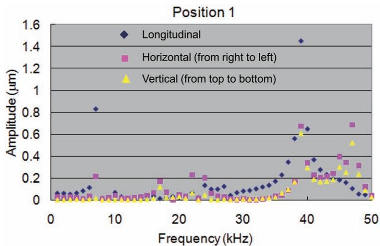
**Fig. 5.** Relation between amplitude and frequency at an applied voltage of 10 V peak-to-peak. Position 1 is the position shown in Fig. 2c, namely, the actuator marked “X” was positioned at the top.
