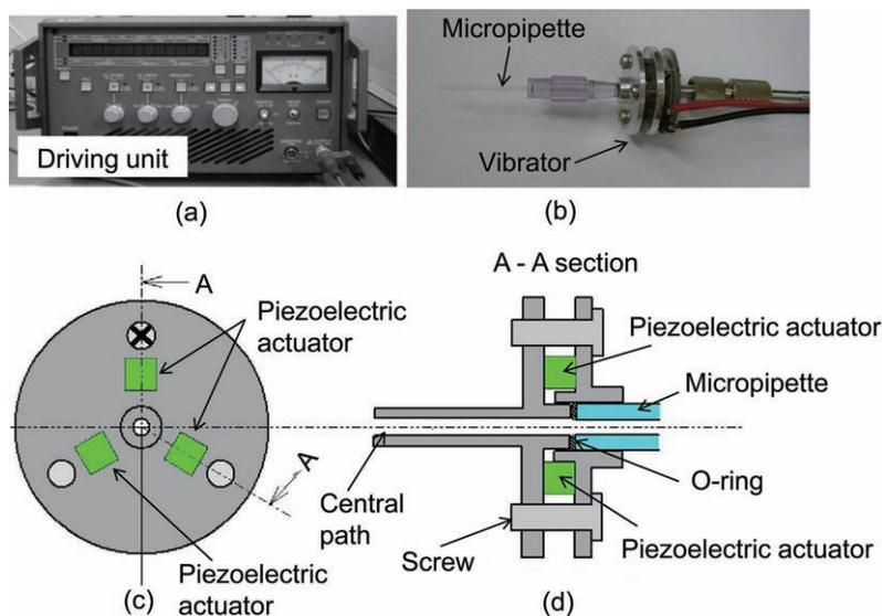
**Fig. 2.** Vibratory microinjection system. (a) the driving unit, (b) the vibrator with a micropipette, (c) front view of the vibrator, (d) side view of the vibrator.
